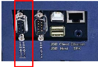
Connector COM2 [RS-232] & COM3 [RS-2422/485]
