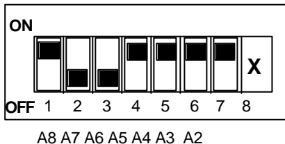
Figure 2.3 Default DIP switch setting
