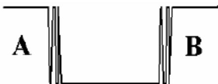
command 02 in A and B position, the response will be that no keystroke has been made and the keystroke information will be lost. In contrast, reading the latched low digital input at DI address **10160** using Modbus command 02 will solve this problem. When issuing 02 command in A and B position, the response denotes that there has been a low pulse between the A and B position indicating a keystroke.
