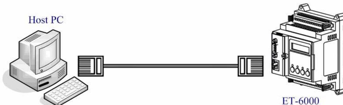
As a result of the automatic MDI / MDI-X crossover for plug-and-play on the ET-6000 RJ45 port, there is no need to a crossover cable to connect the ET-6000 to the Host PC, and only a general straight-through cable is needed to make the connection. The straight-through cable is shown as follows:
