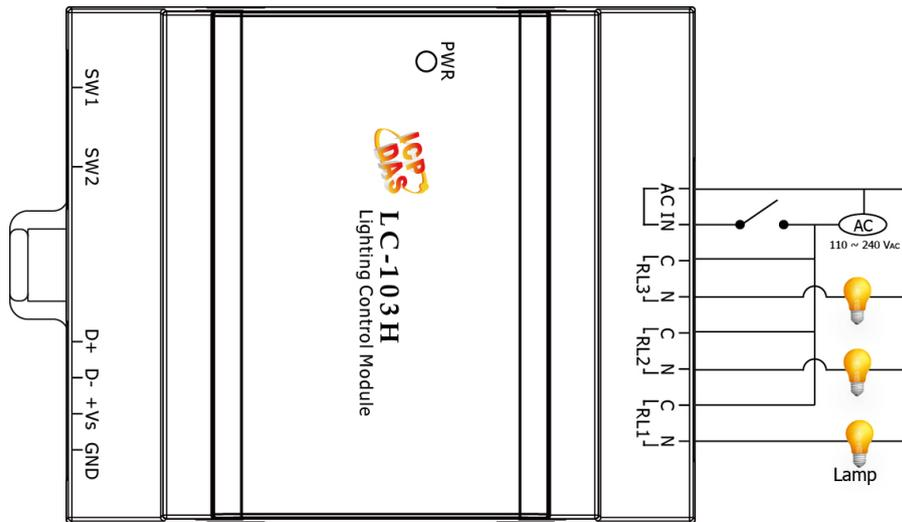
The LC-103H has a single AC input that can be used to connect a lighting control switch and three relay outputs that can be used to connect the lighting, lamp or AC LED lighting etc. Please refer to the above diagram for detailed wire connection information. The input channel of the LC-103H can directly control its 3-channel relay ON and OFF sequence without requiring a remote host controller, so it's very easy to test any lighting circuits for incomplete applications.
