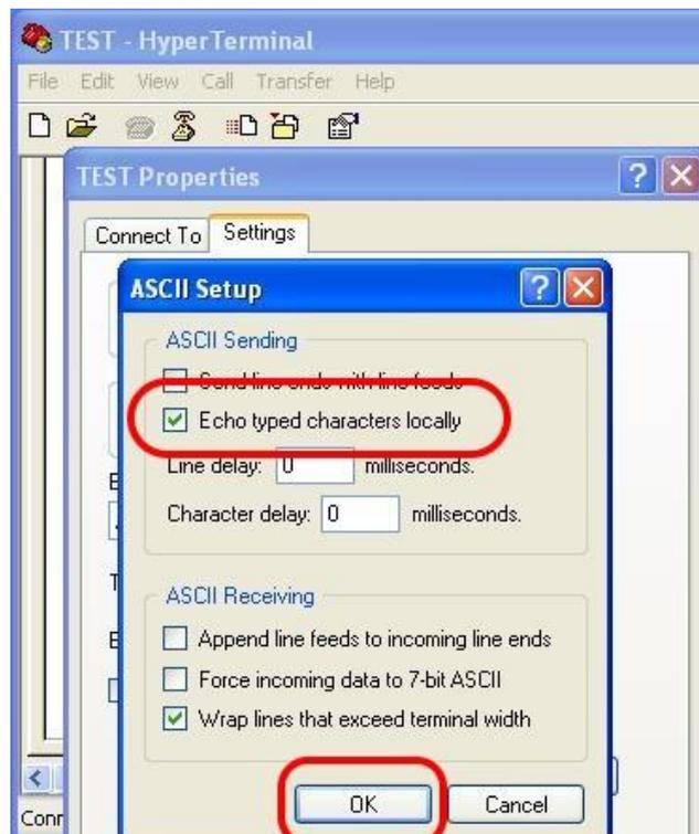
Step9. Input "AT" and press "Enter", then you will receive "AT OK"
