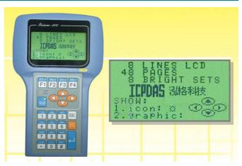
The iVIEW-100 series can be also used as a HMI device for our I-7188 and I-8000 series embedded controller. Since the basic hardware design of iVIEW-100 is similar to that of I-7188 series, all our available software can be used in iVIEW-100. User can design iVIEW-100 application with C Language. We are porting ISaGRAF software PLC to iVIEW-100-ISaGRAF for more programming options and providing iVIEW-100E with a 10/100 mega Ethernet port for internet.
