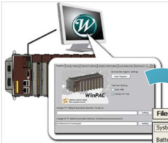
Step 2: Configure IP address (DHCP), FTP Server, Auto Execution files, etc.
