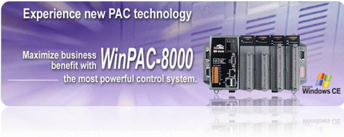
WinPAC-8000 is the second generation PAC of ICPDAS. It equips a PXA270 CPU (520 MHz) running a Windows CE.NET 5.0 operating system, various connections (VGA, USB, Ethernet, RS-232/485) and 1/4/8 slots for high performance parallel I/O modules (high profile I-8K series) and serial-type I/O modules (high profile I-87K I/O modules).
