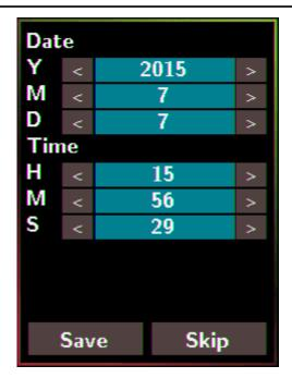
Y: Sets the year from 2000 to 2159 M: Sets the month from 1 to 12 D: Sets the data from 1 to 31 H: Sets the hour from 0 to 23 M: Sets the minute from 0 to 59 S: Sets the second from 0 to 59 Save: Saves the modification and returns to the Settings menu. All the changes take effect immediately after saving changes. **Skip**: Returns to the Settings menu without saving any changes.
