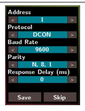
Address: Sets the address for a module.
