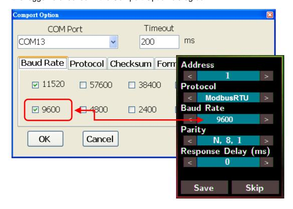
6. Select the Protocol tab and check the protocol that set in the logger.
