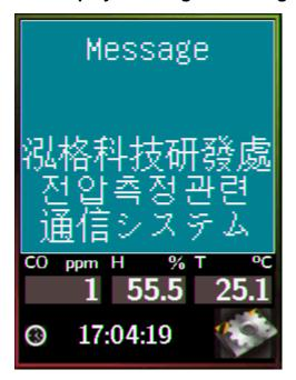
The display message function supports multilingual character sets in UTF-8 encoding. Users can remotely display pre-saved messages or dynamic messages by Modbus commands, or send a dynamic message through the web interface.
