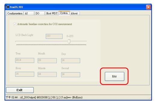
Check/Uncheck the item to Enable/Disable ABC function Set the LCD Back Light (For DL-302 and DL-303 only)
