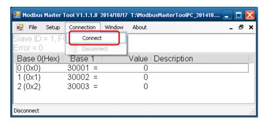
5. Select the communication interface. When using *TCP/IP* as the interface, input the IP for your logger and click on the *OK* button.
