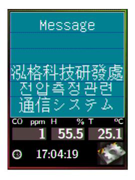
The display-message-on-screen function supports multiple language character sets based on UTF-8 encoding. A message can have a maximum of 6 lines and 14 half-width characters or 7 full-width characters maximum each line.
