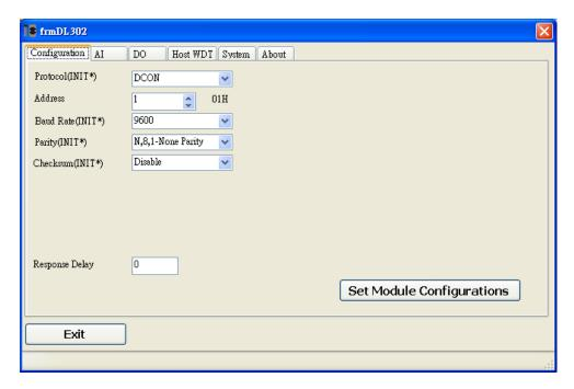
When a DL-300 module is powered-on with the pin 4.INIT in ON position, the protocol is DCON, address is 0, Baud Rate is 9600 bps, Parity is set to N/8/1 and Checksum is disabled.
