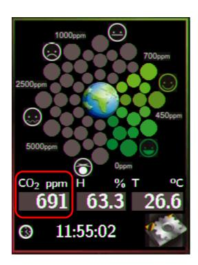
According to the concentration of CO/CO<sub>2</sub> in the air from low to high, the illustration at the center of screen shows from green to red:
