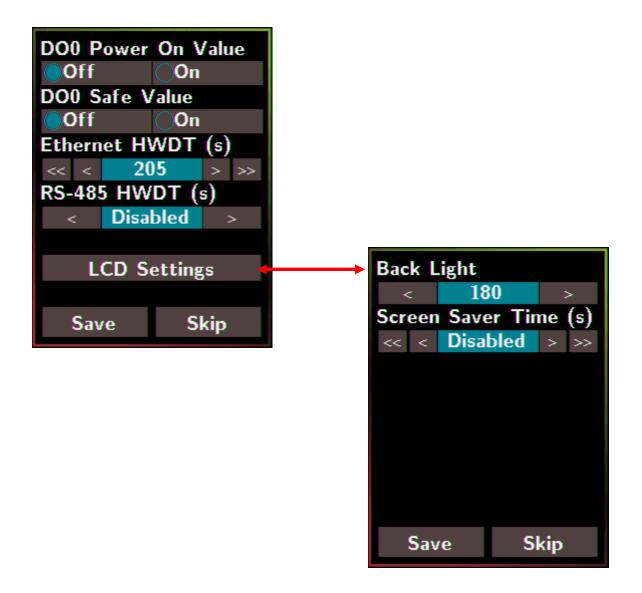
DO0 Power On Value: Sets the relay output status when the DL-300 is powered on. It is invalid when the any one alarm mode for CO/CO₂/Humidity/Temperature/Dew Point in Alarm &Temperature sub-menu is not disabled.
