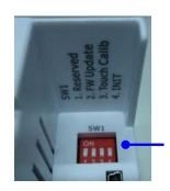
The functions are printed on the top beside the SW1 DIP switch. All the 4 dip switches need be turned to the off position for normal operation.
