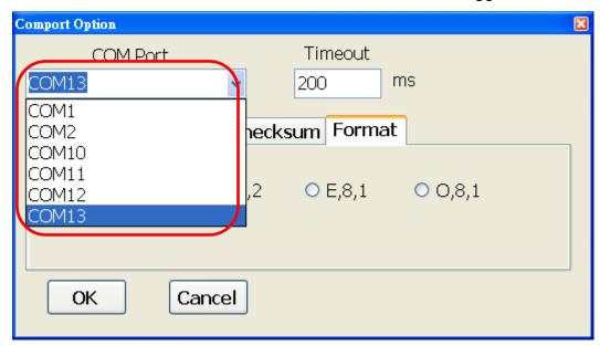
5. The Baud Rate is factory default to 9600 bps, make sure the baud rate setting in the logger is checked in the Comport Option dialog box.
