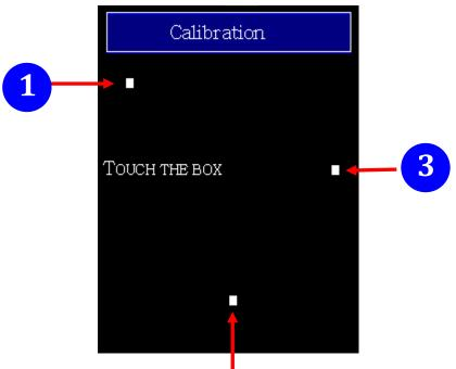
4. Touch one blue box, till the module senses the touch input and sounds. Then touch the next box one by one till the 5 five boxes are sensed.
