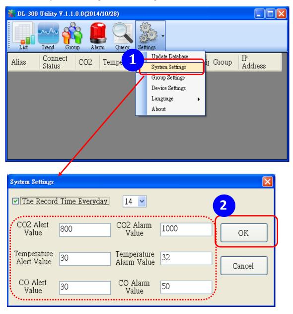
Set the CO/CO2 Alert Value, CO/CO2 Alarm Value (If it is supported in the logger), Temperature Alert Value and Temperature Alarm Value for trigger events. Check the checkbox next to The Record Time Everyday can schedule auto generate report everyday at the time set in the dropdown menu. Click on the **OK** button to complete the settings.
