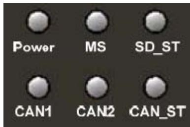
Figure 2-7 LED Assignment of CAN-Logger200
