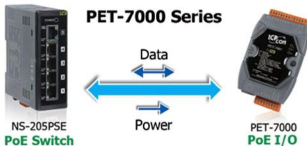
When using PET-7016 module, you can choose ICP DAS “PoE” switch – “NS-205PSE” as the power source, NS-205PSE automatically detects the connected devices whether they are PoE devices or not. This mechanism ensures NS-205PSE to work with both PoE and non-PoE devices coordinately at the same time.
