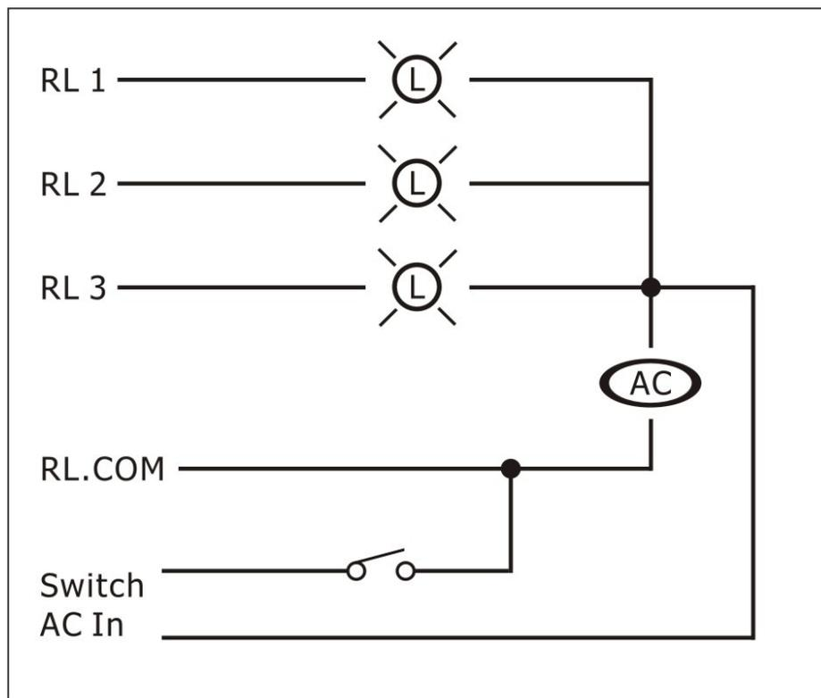
The LC-103 has a single AC input that can be used to connect a lighting control switch and three relay outputs that can be used to connect the lighting, lamp or AC LED lighting etc. Please refer to the above diagram for detailed wire connection information. The input channel of the LC-103 can directly control its 3-channel relay ON and OFF sequence without requiring a remote host controller, so it's very easy to test any lighting circuits for incomplete applications.
