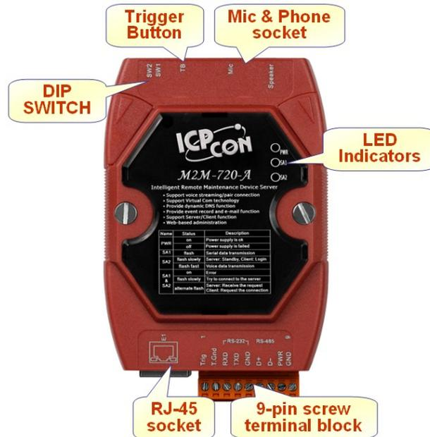
Figure 3: Pin assignment of M2M-720-A
