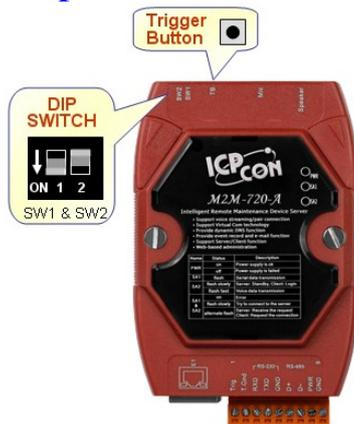
**Step 4: M2M-720-A's IP should be returned to "192.168.1.217". Please set PC's Network settings. The settings must have the same domain and different IP with the M2M-720-A (ex: IP=192.168.1.210, mask=255.255.255.0).**
