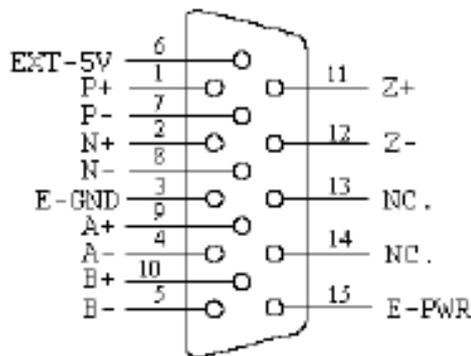
Fig. 3-8 Pin definition for CN5 ~ CN8
