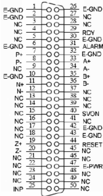
Fig. 3-5 Pin definition for CNX, CNY, CNZ, CNU
