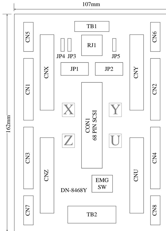
Fig. 3-1 Board layout for the DN-8468YB
