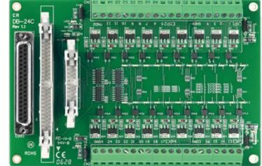
The transistor is energized by applying a 5-voltage signal to the appropriate input channels on the 50-pin header or 20-pin header or 37-pin D-sub connector. Twenty-four enunciator LEDs, one for each transistor, light when their associated transistor is activated. The DB-24C daughter board is connected to the CN1/CN2 connector on the card using a 20-pin flat cable.
