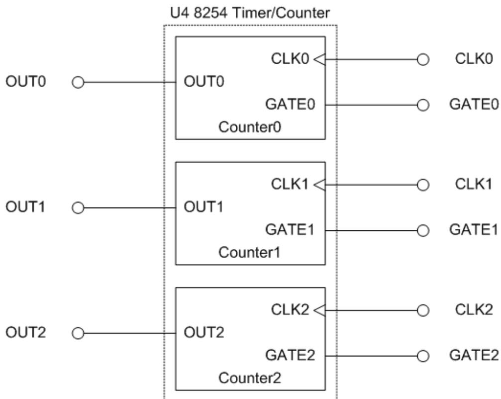
The second 8254 chip is used to generate interrupt trigger signals, as shown in Figure 2.5. The Counter3 accept event signal and will generate trigger signal of the interrupt. And the Counter4 and Counter5 are cascaded together, which has clock source 4 MHz. It is used to generate pacer timer trigger of the interrupt.
