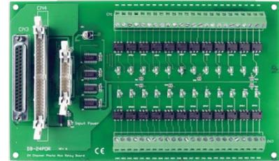
The relay is energized by applying a 5 voltage signal to the appropriate relay channel on the n the 50-pin header or 20-pin header or 37-pin D-sub connector. Twenty-four indicators LEDs, one for each relay, light when their associated relay is activated. The DB-24POR daughter board is connected to the CN1/CN2 connector on the card using a 20-pin flat cable.
