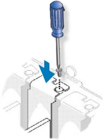
**Step 9:** Confirm that the board is correctly inserted in the motherboard, and then secure your board in place using the retaining screw that was removed in Step 6.
