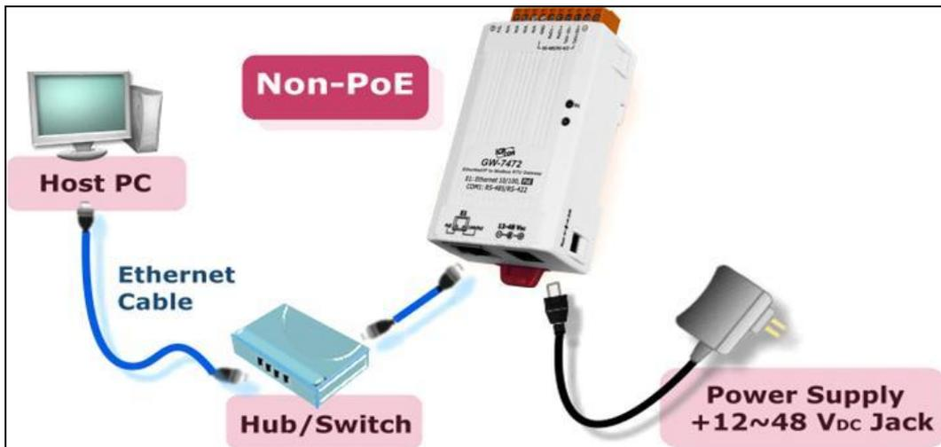
Figure 3.1 GW-7472 with DC jack power supply
