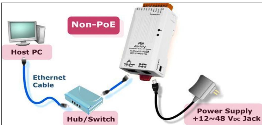
Figure 3.4 GW-7473 with DC jack power supply
