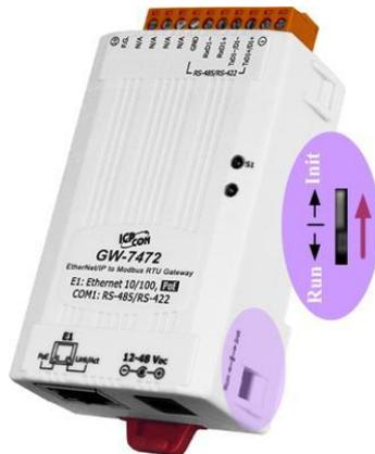
In Init mode, the GW-7472 is forced to the network configuration as following table. Connect the GW-7472 with your computer at the same sub network or by using the same Ethernet switch. Then power the GW-7472 on. Afterwards, you can use the command “ping 192.168.255.1” in the Command Prompt window to test if the connection between the GW-7472 and your computer is OK.
