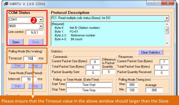
Please ensure that the Timeout value in the above window should larger than the Slave timeout setting in the tSH-700 series module.
