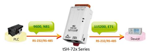
Modbus RTU/ASCII Conversion: This function allows a single Modbus RTU/ASCII master device to communicate with Modbus RTU/ASCII slave devices using different protocols, baud rates and data formats.
