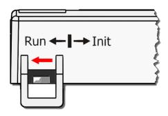
**Step 4** Reset the Init/Run switch on the tSH-700 module to the "Run" position and reboot the device.
