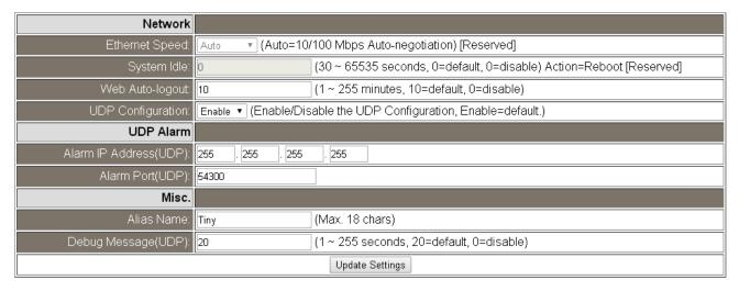
The following is an overview of the parameters contained in the **General Settings** section:
