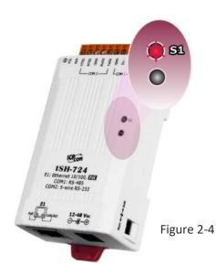
5. Verify that the System LED indicator is flashing.
