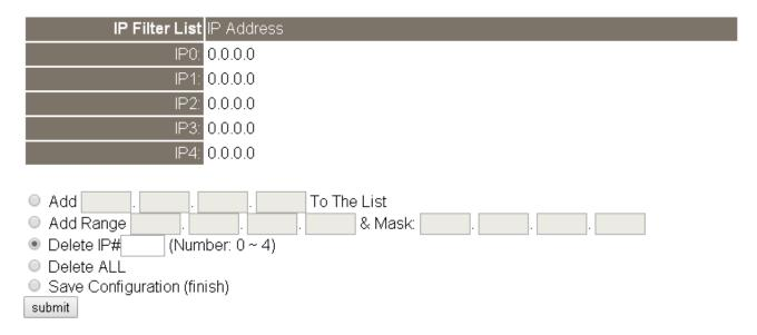
The following is an overview of the parameters contained in the **Accessible IP (filter is disabled when all zero)** section:
