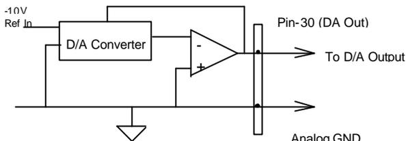
The operation of D/A conversion is simpler than A/D operation. You only need to write digital values into the D/A data registers and the corresponding voltage will be output from the DA Out (pin-30 of CN3). Refer to section 3.15 for information about the D/A data registers. The mathematical relationship between the digital data  $DAn$  and the output voltage is formulated as following:
