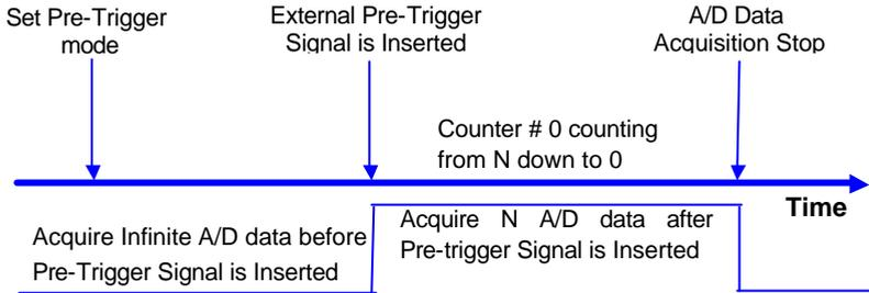
If the application acquires data after the pre-trigger signal, only the last N data need to be stored. The maximum value of N is 65535. If the application only needs to acquire data before the pre-trigger signal, set N=1 then just one more data will be sampled after pre-trigger signal and infinite data before pre-trigger signal can be stored.
