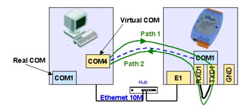
Step 3: Virtualize 7188E/8000E's COM1 to become PC's COM4 by using the VxComm Utility.
