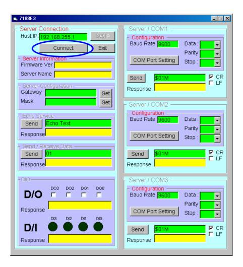
Step2: Press "Connect" button. The program will then readout relative information concerning the 7188E3 and start scaning the DI of the7188E3.
