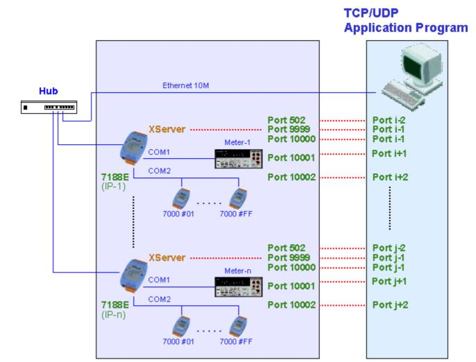
The Xserver is a powerful program designed for Ethernet I/O appllications. It supplies the 7188E with a range of flexible options. Users can modify the Xserver to control all of the 7188E's hardware: COM ports, I/O expansion boards, a 7 Seg LED, or other relevant products.
