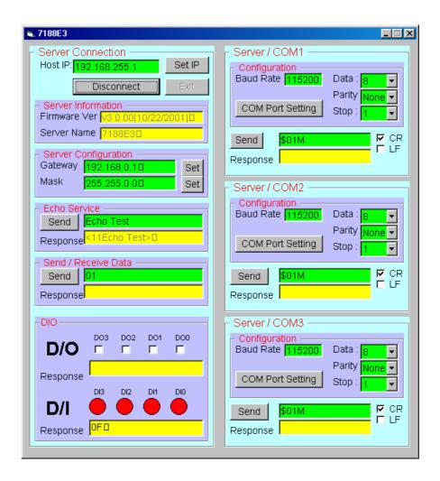
Step 3: Send "10" to readout the module name.
