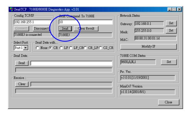
Step 4: Select "Port 2" and "CR". Then send "\$02M" to read 7000 module's ID which is connected to 7188E3's COM2. If you enable 7000 module's checksum function, select "CS\_CR". The "CS\_CR" option will add two checksum bytes, then adds "CR".
