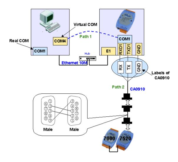
Step 3: Click the menu item "COM Port" to choose the COM port number, baudrate, and checksum. For example: COM10, 115200, 19200, 9600 and No-Checksum. (These settings depend on the 7000 series module's settings.)
