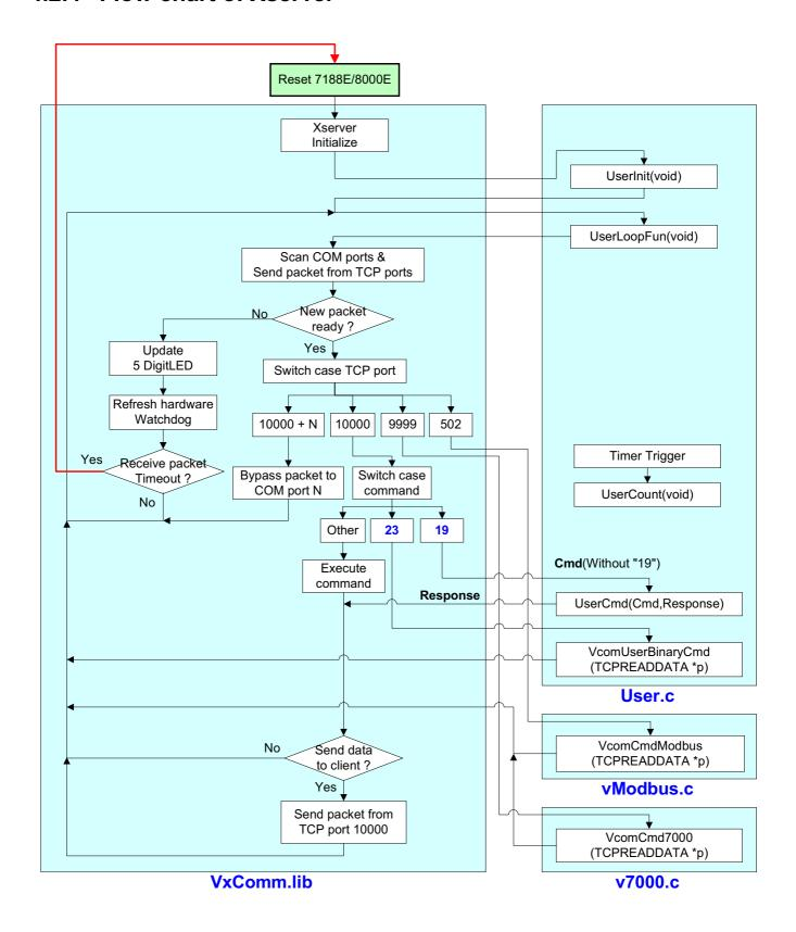
It is very difficult to develop an enbedded controller program with Ethernet/Internet communication. But by using the Xserver, users can do that quickly and easily. Users need only modify 7 functions in User.c, vModbus and v7000.c. Users build their own code in the 7 functions to make the Xserver work as they desire. The features of the 7 functions are listed below:
