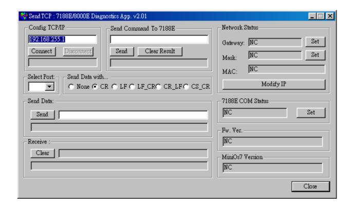
Step 2: Press "Connect" button to connect to 7188E3.
