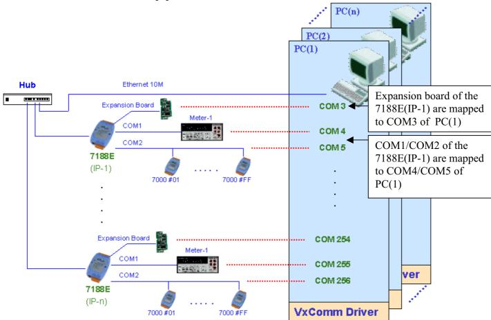
To use the Virtual COM application, first install the VxComm Driver. After installation, the VxComm Utility can map any 7188E's remote COM port. These virtualized COM ports can be used by the PC to control devices directly, just as you would use COM1 (real COM port) to control devices. When using the Virtual COM application, one PC can use a maximum of 256 COM ports. Users need not worry about network connections. The VxComm Driver will handle all Ethernet/Internet connections.
