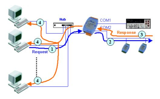
Condition 2: No clients send a request to Xserver to access devices. The Xserver echoes data from devices to every client which are connected to the 7188E/8000E.
