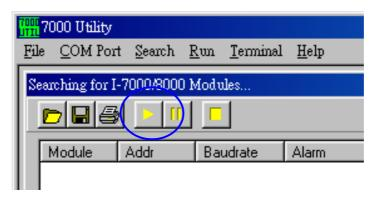
Step 5: If the VxComm Driver works well, the 7000 Utility can search the module(s) connected to the 7188E/8000E's COM1.
