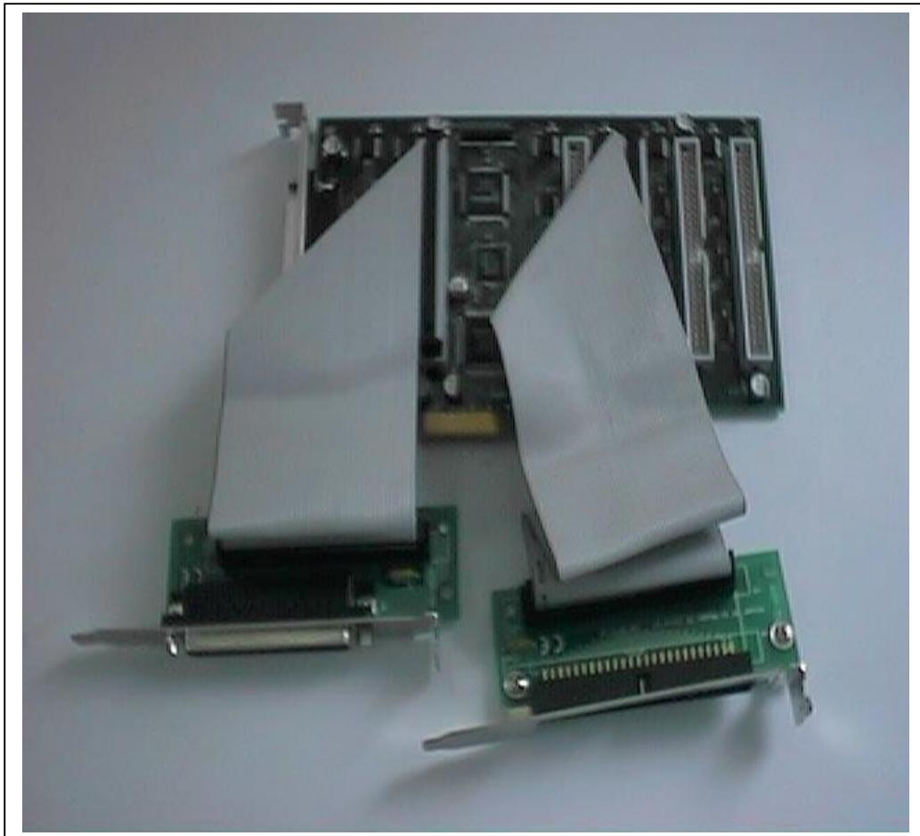
ADP-37/PCI: 50-pin header to DB-37 extender.
