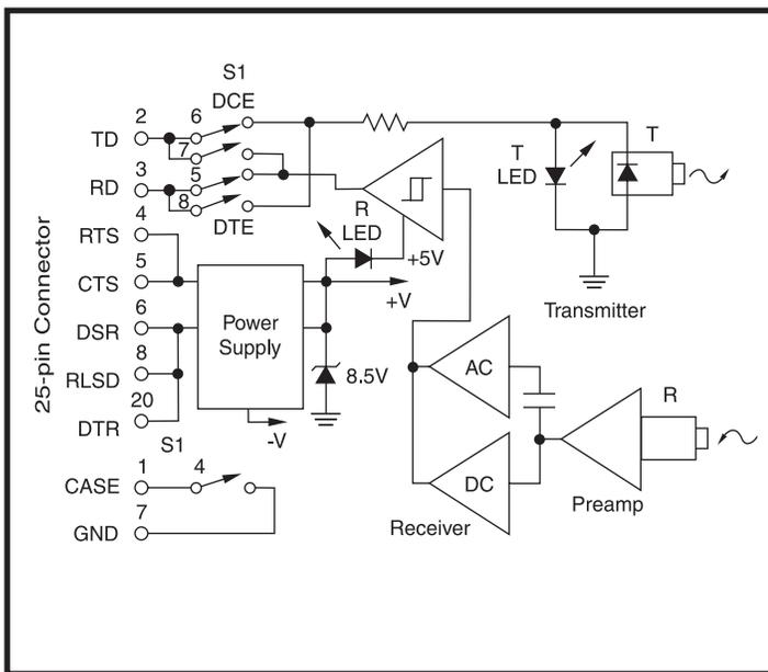
Figure 1: LDM80 Block Diagram
